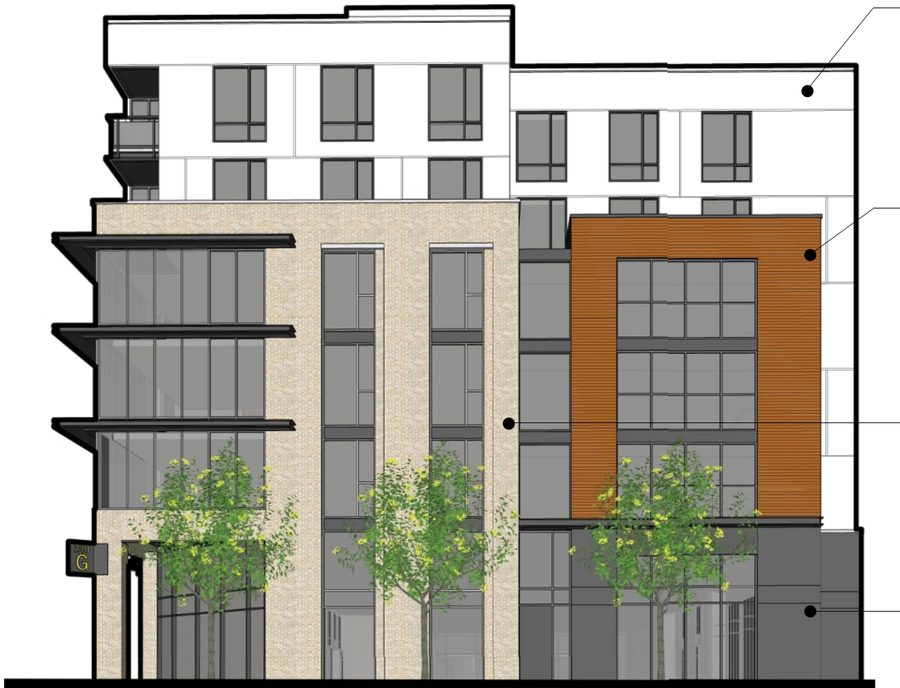
White Planes: Portland Cement Plaster Color: White Texture: Smooth
